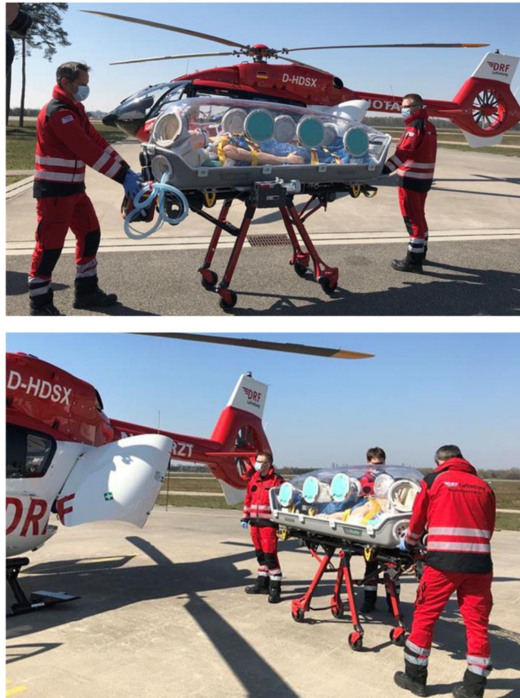
Fig. 2 The EpiShuttle® of the DRF-Luftrettung (©DRF-Luftrettung – Germany). The EpiShuttle is used only for interfacility transport. It is fitted into the helicopter (EC 145 / H 145) before the mission. The DRF-Luftrettung has an exemption according to article 71 (1) of regulation (EU) 2018/1139 by the “Luftfahrt-Bundesamt – LBA” (civil aeronautics board of Germany) to use the EpiShuttle in the Eurocopter 145 and Airbus Helicopter 145 rotor wing aircrafts of the company
