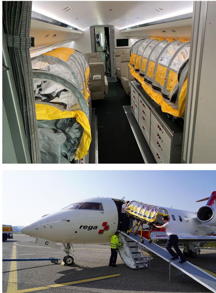
Fig. 3 PIU owned by the REGA (©REGA - Switzerland). The REGA PIU is mainly used in the fixed wing aircrafts (Challenger 650) of the company. Transport of 2 PIU per flight are possible in the Challenger 650
